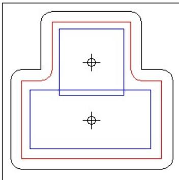
Two G-code files are needed to machine the Pocket.
